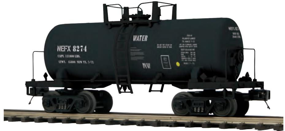
Maintenance of Way (Non-Potable Water) - 8000 Gallon Tank Car
